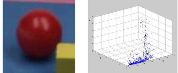
Figure 1: Color distributions for a red ball. The superimposed arrow indicate the illuminant color. The color distribution can be easily separated in a body reflectance part and a part in the specular reflection part in the illuminant direction.
